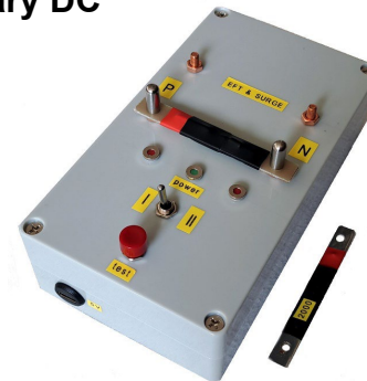
Simulator of Equipment that Needs to be Protected by EMI/HEMP Filters
