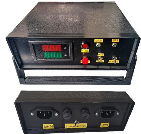
UPS and Static Switch Tester for Express Test
